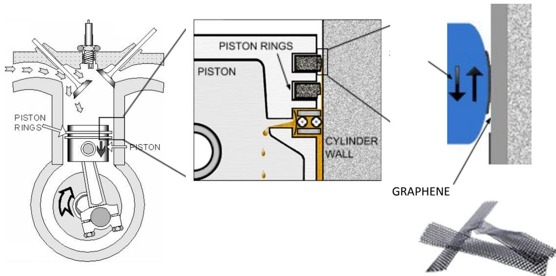
Graphene as lubricant additives bond to metallic surfaces to keep moving parts physically separated under loads, high temperatures and speeds, thus minimizing friction and wear.
